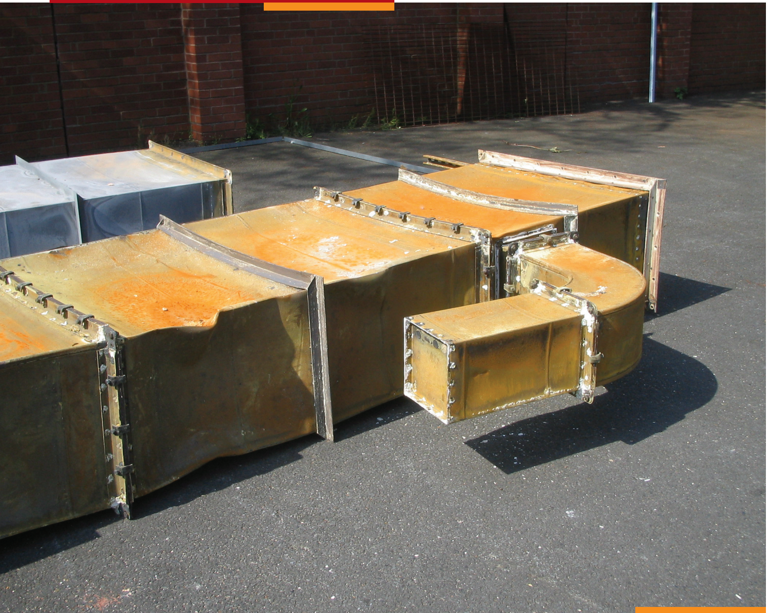
Duct (A) cooled down after a 2 hour test at 1100 Degrees C. Shows limited distortion
